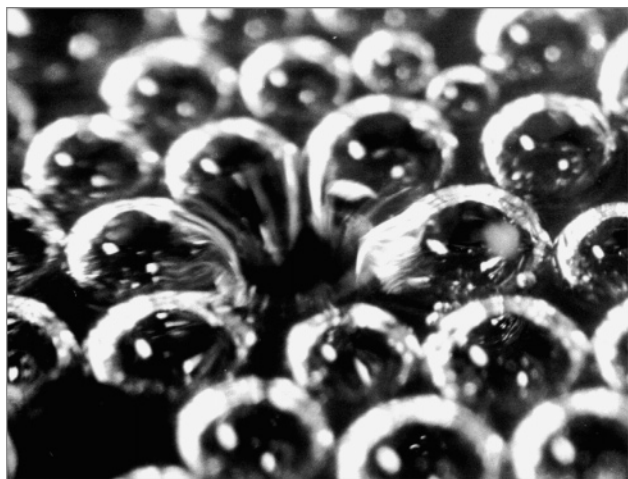
Figure 22. Oblique view of a bursting event in a bubble raft composed of quite monodisperse millimetric bubbles. Bar = 1 mm.
